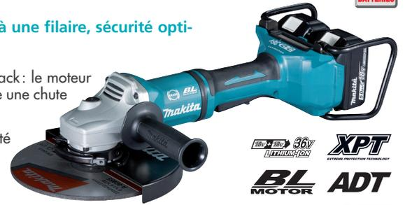
36 V => 2x 18 V Li-Ion 5 Ah, 6000 tr/min, Prise en main Ø 160 mm, Ø 230 mm, M14 mm, Pression sonore (Lpa) 88 dB(A), Dimensions (Lxlxh) 462x250x156 mm, Poids net EPTA 5,2 kg.
